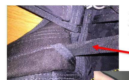
Start by checking the routing and stowage of the ACE RSL LANYARD. Be sure that the lanyard is clear and free and the ring has a direct line to the reserve cable and guide rings. The lanyard should exit the RSL sleeve at the top of the yoke with the ACE Air Snare on the rear.
