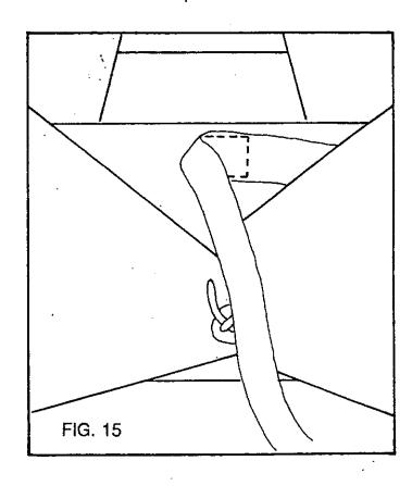
15a) [For pilot chute pouch on right leg strap]. Mate the velcro on the bridle to the velcro track provided near the lower edge of the right side flap. This will lead the bridle along the container to the harness near the mouth of the pilot chute pouch. There will be some slack in the bridle between the curved pin and the velcro track. Tuck this slack up under the lower edge of the right side flap as shown in FIG. 16. (Skip Step 15b and go to Step 16.)
