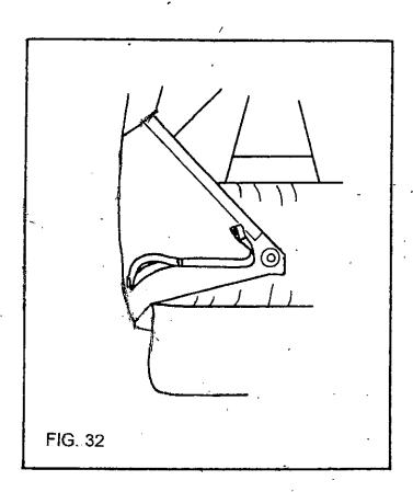
1) To install the Left Yank, mate it to the velcro track on the middle of the left main side flap before closing the main container (FIG. 32). The large loop (the grip) is to the left, and the small loop is closest to the grommet of the left side flap.
