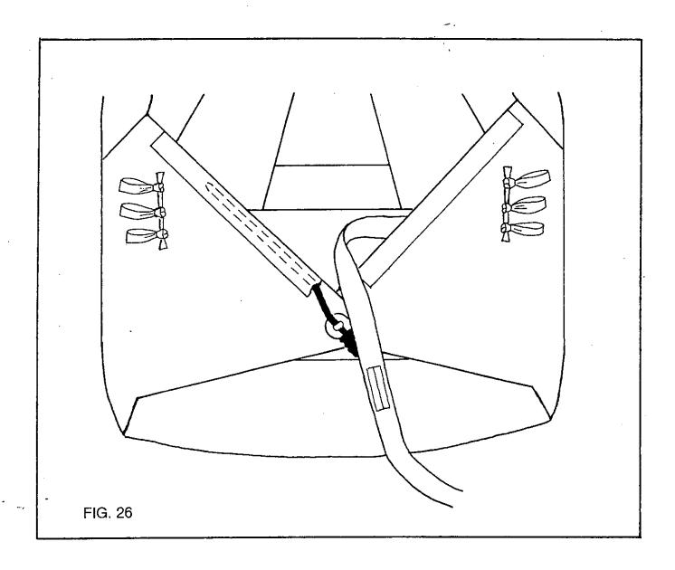
14-a) There is an "excess cable channel" along the upper edge of each main side flap. After the cable is inserted thru the closing loop, the excess length may be stowed in one of these channels as shown in FIG. 26.
